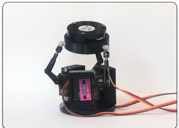
Stewart Platform (3DOF) Designed, implemented, and photographed by Abena
